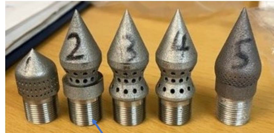
3d-printed variants of umbrella plume 3d-printed copy of original
